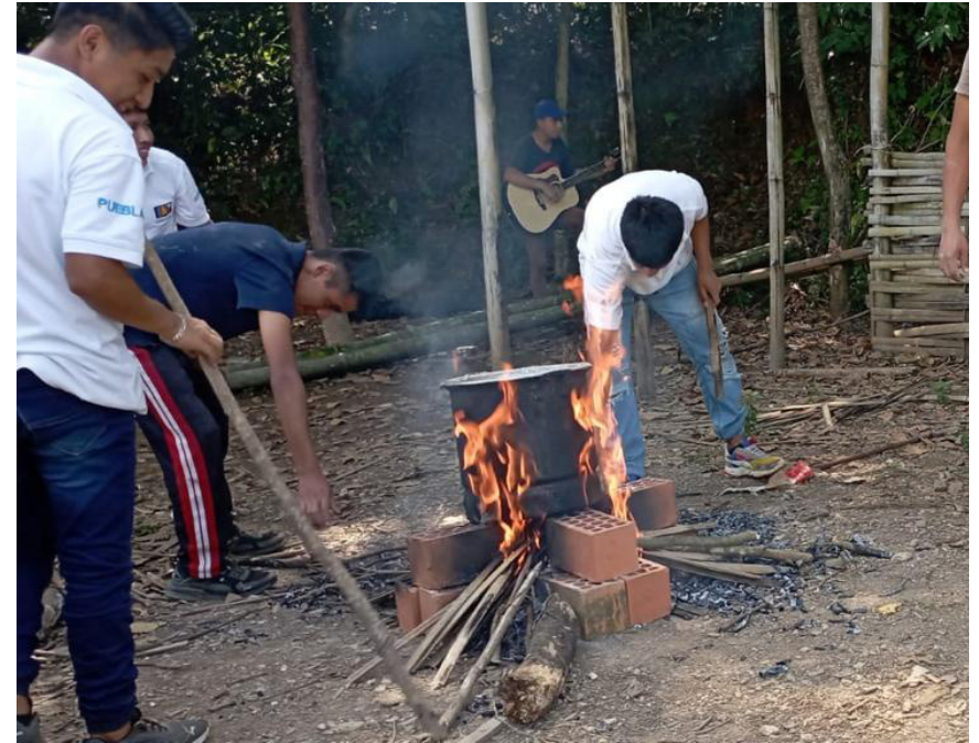
Technical training and student input: Mixing chemicals for bamboo preservation. Photo: Community of students and teachers.
