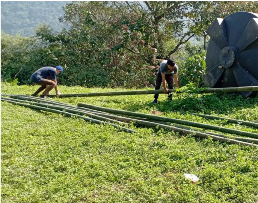
Technical training and student input: Cleaning bamboo before treatment. Photo: Community of students and teachers.
