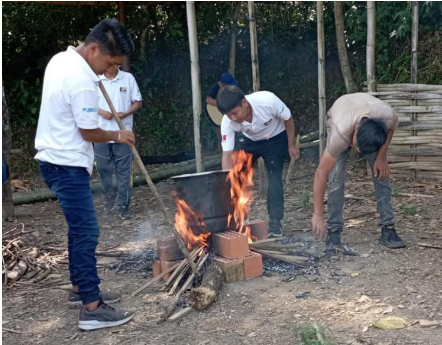
Technical training and student input: Mixing chemicals for bamboo preservation. Photo: Community of students and teachers.
