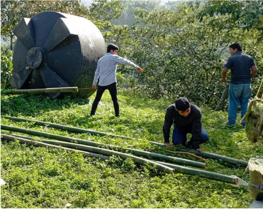
Technical training and student input: Cleaning bamboo before treatment. Photo: Community of students and teachers.
