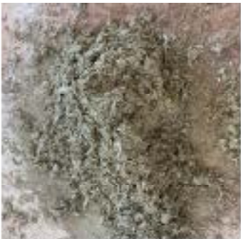
Step 4: Adding the clay slurry to the dry mix.
