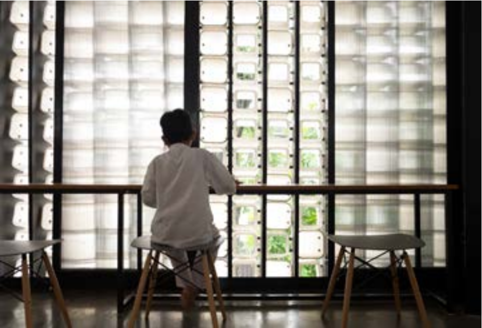
Microlibrary Bima utilizes 2,000 secondhand ice cream buckets as a performative façade, effectively filtering daylight and facilitating natural ventilation. Photograph by Sanrok Studio, 2016
