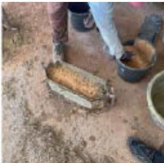
Step 6: Adding sand to the compacted mix before removing from the mold.
